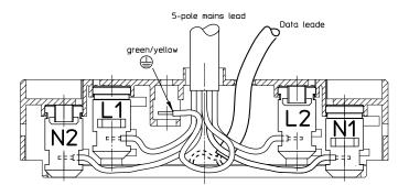
When wiring the track, check that the earth conductor(green/yellow)and the neutral conductor (blue)are connected, as indicated in the illustration.
